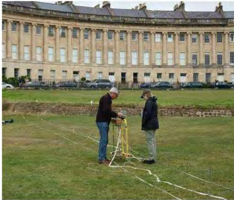
Profiling - Electrical Resistivity Tomography (ERT)
